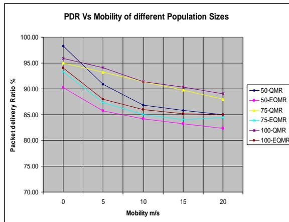
**Fig. 3** Packet Delivery Ratio vs. Mobility for different population size
