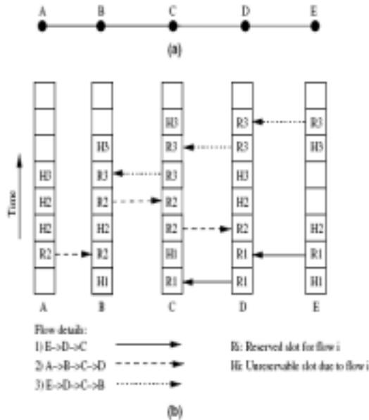
Fig. 2 Illustration of MBR scheme: (a) example network topology and (b) MBR scheme.
