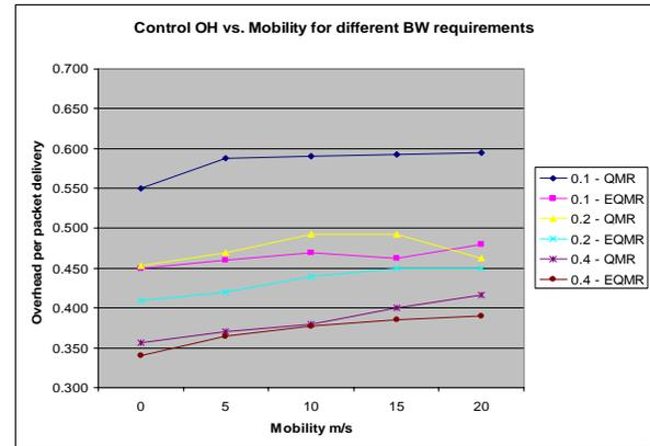
**Fig. 6 Control OH vs. mobility for different bandwidth requirements**
